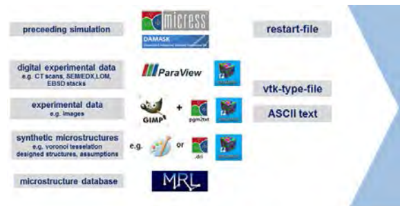
Figure. 2: The “initial conditions” entering a microstructure simulation as initial microstructure may originate from a variety of sources. A similar variety of software tools serves the other arrows being depicted in fig. 1 [6]
